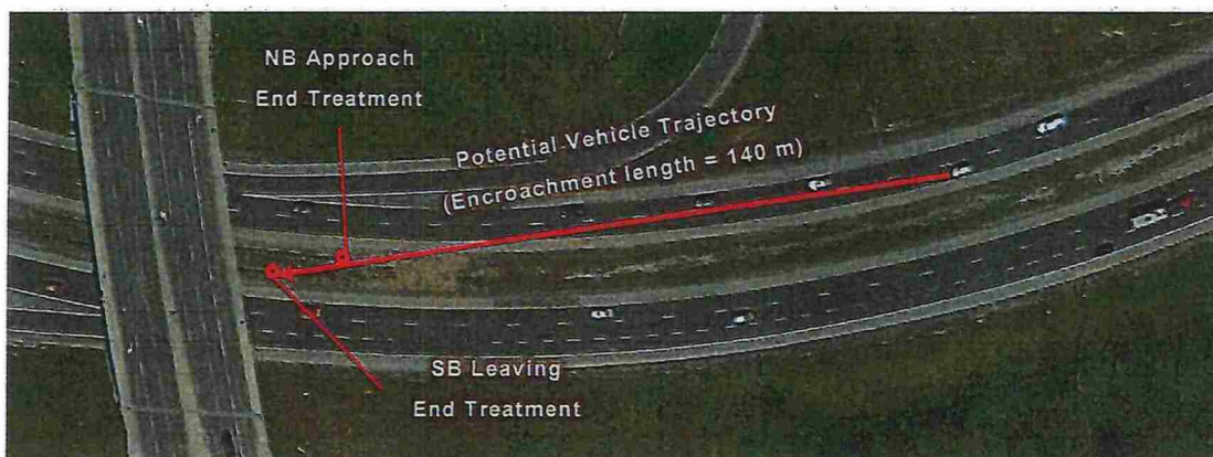
Figure 19: Potential trajectory of a vehicle towards fishtail end treatment
