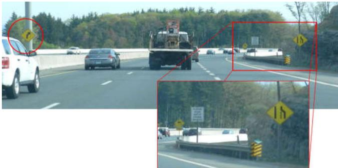
Figure 23 - Closely Spaced Signs within the Vicinity of a Complex Merging Area (View North from the Mainline)
