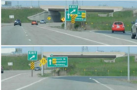
Figure 25 - Closely-Spaced and Eclipsing Signage (View West from Beginning of On-Ramps)
