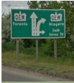
Figure 35 - Example of Diagrammatic Sign.
