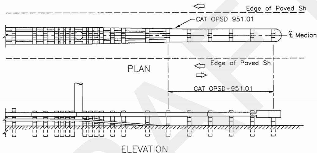
Figure 32: Steel beam protection of structures located on the median<sup>31</sup>
