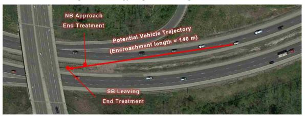
Figure 19: Potential trajectory of a vehicle towards fishtail end treatment
